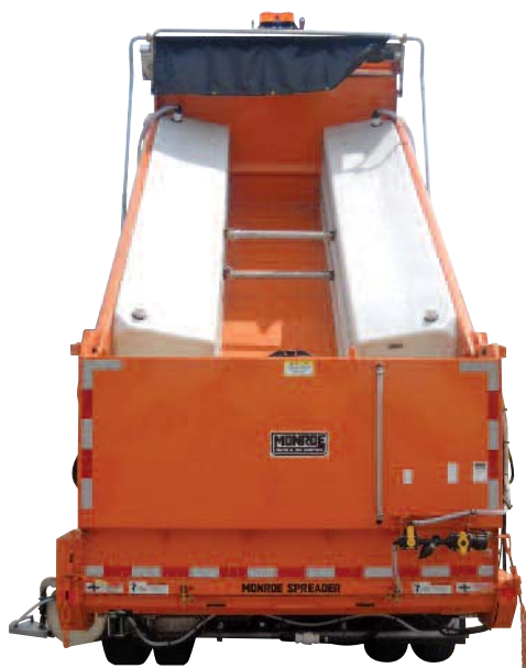
In-Bed Tank Pre-wet System
